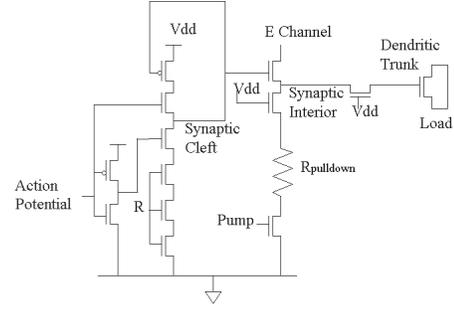
Fig. 1. The Carbon Nanotube Synaptic Circuit
